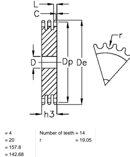
C = 4 D = 20 De = 157.8 Dp = 142.68 For chain size = 1  $1/4 \times 3/4$ For chain type = 20 B-3 h3 = 91 L = 18.2
